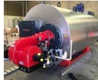
Industrial Package Boiler
