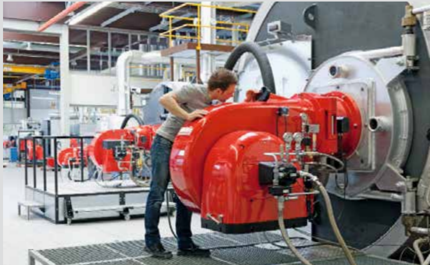
Test-firing chambers for medium and large-sized burners at the Weishaupt Research & Development Centre
