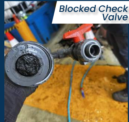
Waste Blockage Cleared From Drainage Chamber
